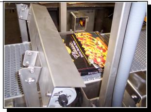
The Pass or Fail state from one of the three inspection points, determines whether the PLC will
